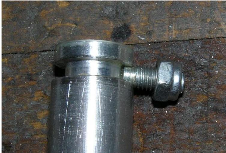
These photos show the principle of the turnable lower lever part. The fixing screw engages in the groove of the lower lever and fix it axially.
