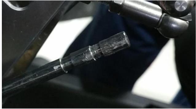
remove the plastic rope completely; smooth filing the ribbing until the ball fits about
