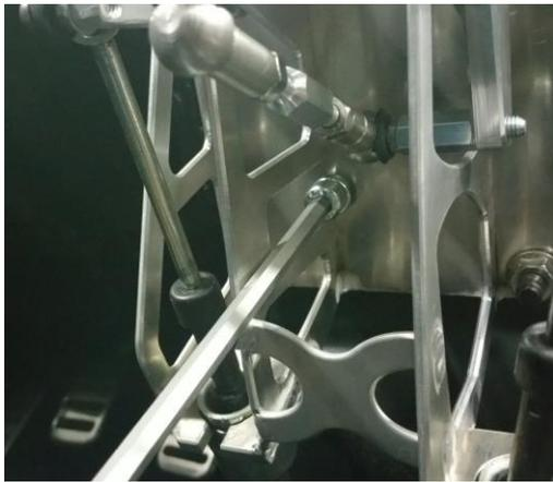
tighten the Shifter with 3 hex nuts and 1 inbus screw
