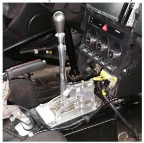
This unit is designed for racing vehicles without interior and center console. Retained Center console must be modified to allow the necessary free movement and installation for the shifter. The base of this unit must be screwed directly onto the sheetmetal of the center tunnel.
