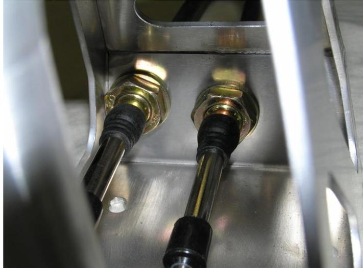
To mount the nuts take off the rubber boot, then the nuts can be mounted easily. The cable with length=1150mm is the selection cable and has to be mounted in driving direction left side. The shorter one (length=1020mm) is the shift cable and has to be mounted in the middle.
