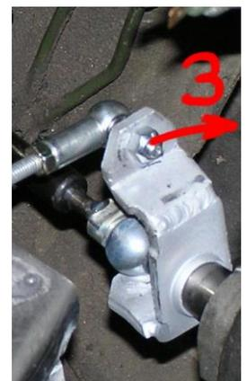
In middle position the gearshift should be slightly turned to the right.
