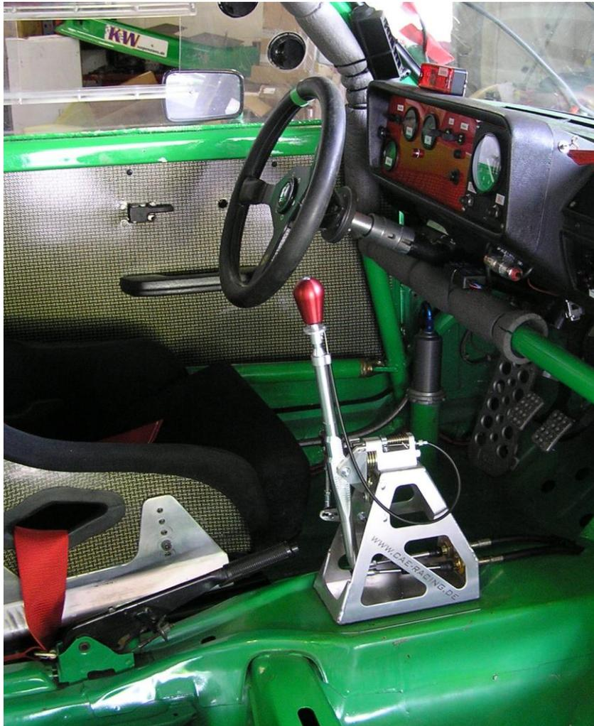
The shifter is intended for Racing Cars without interior equipment. If center console is mounted, it must be dismantled or modified to achieve an acceptable space for the cables. The new unit should be mounted directly on to the floorboard, so part of the carpet must be removed.
