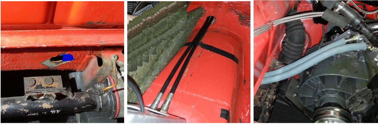
Before drilling you must check if the cables have enough space. If not, change position of holes as far as necessary.
