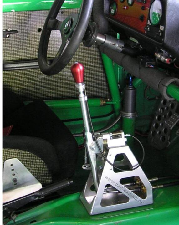
The shifter is intended for racing cars without interior equipment. If center console is mounted, it must be dismantled or modified to achieve an acceptable space for the cables. The new unit should be mounted directly on to the floorboard, so part of the carpet must be removed.
